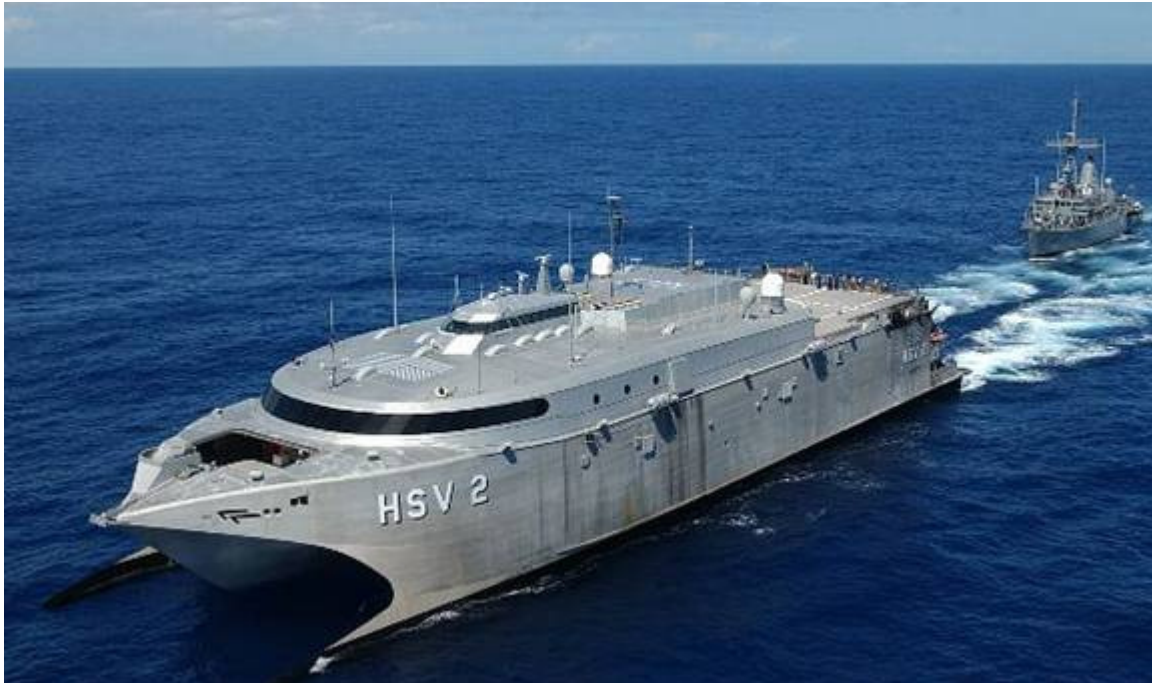
High Speed Vessel SWIFT (HSV 2), an aluminum-hulled catamaran. U.S. Navy photo by Photographer's Mate 1st Class Michelle R. Hammond
